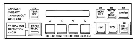
**POWER** (green): On when the printer is turned on and
